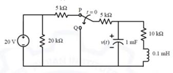
The switch is closed at t=0 while the capacitor is charged to -5 V.(i.e Vc(0) = -5V)
