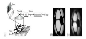
Figure 2: (a) Single-pixel, compressive sensing camera. (b) Conventional digital camera image of a soccer ball. (c)  $64 \times 64$  black-and-white image xb of the same ball (N = 4096 pixels) recovered from M = 1600 random measurements taken by the camera in (a). The images in (b) and (c) are not meant to be aligned.
