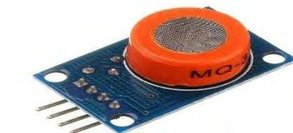
**Fig 5: MQ3 Sensor**
