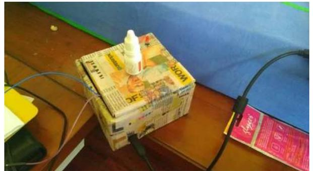
Fig 4: Smart Medicine Box- System is active and waiting for the time of medicine to be taken. LED is turned off.
