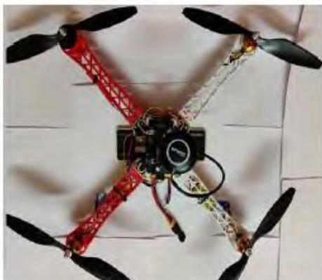
To determine plant health, our quadcopter captures images of the fields/ area and processes them via VARI algorithm. The program outputs a value between 0 to 1; 0
