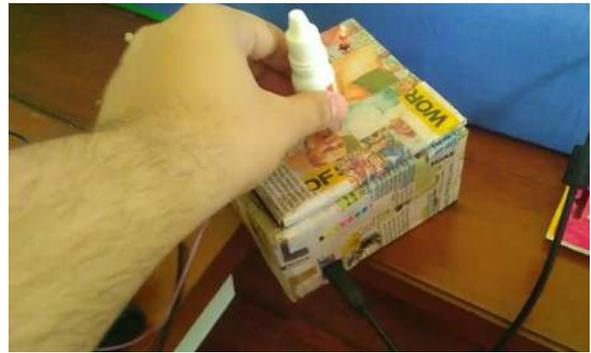
Fig 6: Smart Medicine Box- As the patient lifts the medicine for intake; the LED will glow continuously until medicine is kept back on place. The system will then again until the next time arrives
