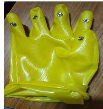
Fig4. Glove and the Metallic buttons
