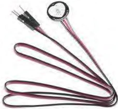
Fig 1.4 Pulse Sensor
