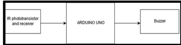
Fig.1: Block Diagram
