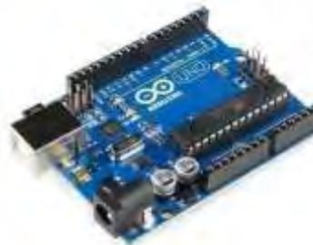
microcontroller and developed by Arduino.cc. This board consists of sets of digital and analog input/output pins that may be interfaced to various expansion boards and other circuits.
