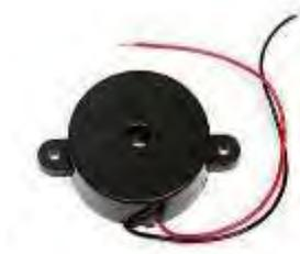
Fig.3.5 Piezo buzzer
