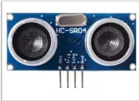
Ultrasonic sensors work by radiating sound waves at a recurrence unreasonably high for people to hear. They at that point trust that the sound will be reflected back, figuring separation dependent on the time required. This is like how radar quantifies the time it takes a radio wave to return in the wake of hitting an article.
