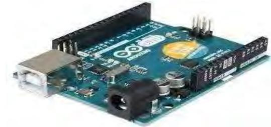
**Fig 3: Arduino Board**
